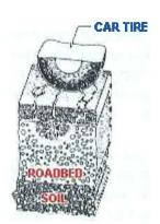
Rainwater sinks through cracks in old or weakened asphalt. The water is soaked up by the mixture of rock, gravel, and sand that supports the road.
