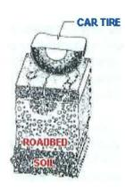
the road force water through the soggy roadbed, eventually eroding parts of it.
