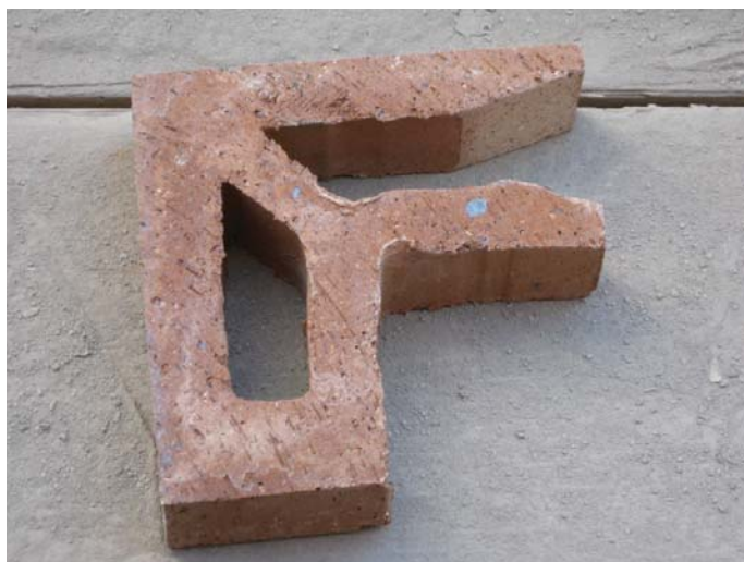
Figure 6 Custom Lintel Unit for an Inset Window
