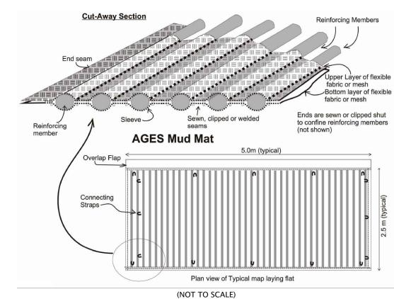
AVOID LOCATING ON STEEP SLOPES OR AT CURVES IN PUBLIC ROADS. REMOVE ALL VEGETATION AND OTHER OBJECTIONABLE MATERIAL FROM THE FOUNDATION AREA, AND GRADE AND CROWN FOR POSITIVE DRAINAGE.
