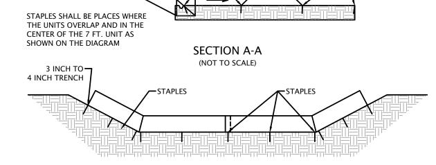
POINT "2" TO ENSURE THAT WATER FLOWS OVER THE DIKE AND NOT AROUND THE ENDS
