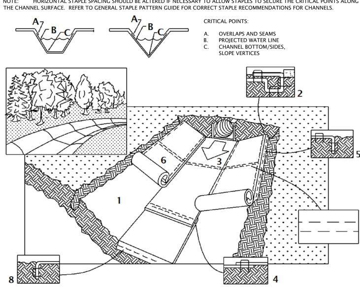
PREPARE SOIL BEFORE INSTALLING BLANKETS, INCLUDING APPLICATION OF LIME, FERTILIZER AND SEED. BEGIN AT THE TOP OF THE CHANNEL BY ANCHORING THE BLANKET IN A 6-INCH DEEP BY 6-INCH WIDE TRENCH, BACKFILL AND
