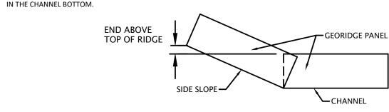
4. THE SPACING IS CALCULATED BY DIVIDING THE HEIGHT OF THE GEORIDGE BY THE GRADIENT OF THE CHANNEL SLOPE. 9-INCH / 0.0.2 GRADIENT = 450 INCHES OR 37.5 FEET
