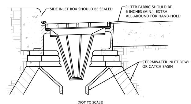
INSPECT AFTER EACH STORM EVENT REMOVE BUILT-UP SEDIMENT AND REPAIR (OR REPLACE IF NECESSARY) THE GEOTEXTILE FABRIC AFTER EACH STORM EVENT. PERIODICALLY REMOVE SEDIMENT AND TRACKED-ON SOIL FROM THE STREET (BUT NOT BY FLUSHING WITH WATER) TO REDUCE THE SEDIMENT LOAD ON
