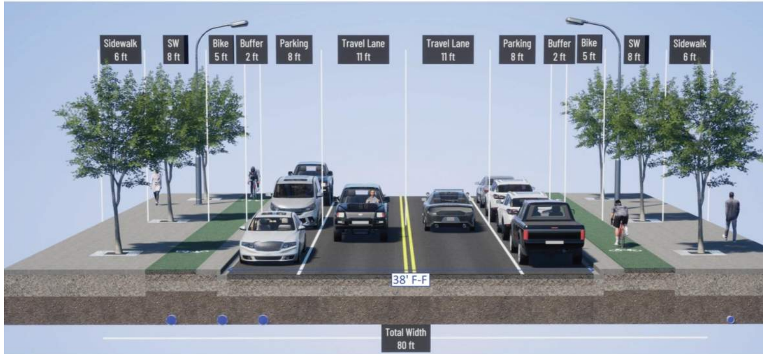
Alternative 1A: 21 ft Raised Sidewalk/Bike, 8 ft Parking, 11 ft Travel Lane
