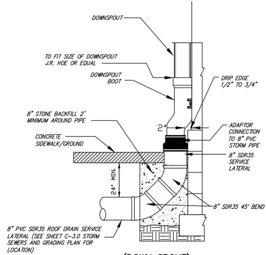
(DOWN SPOUT) ROOF DRAIN PIPE CONNECTION
