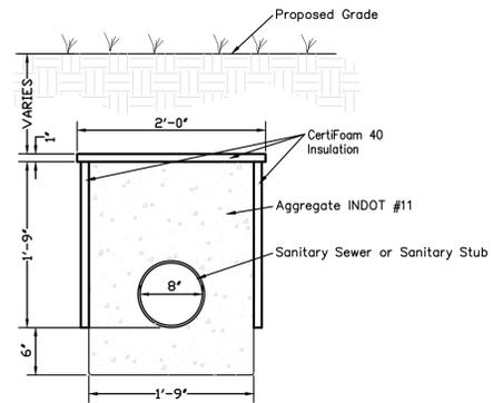
SANITARY PIPE INSULATION DETAIL
