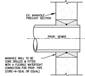
PIPE CONNECTION DETAIL TO EXISTING MANHOLE
