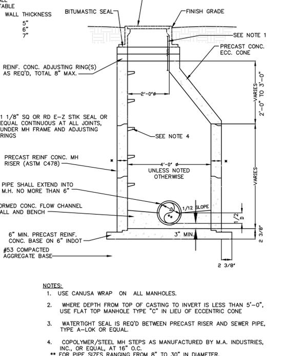
SANITARY TYPE "A" MANHOLE NOT TO SCALE
